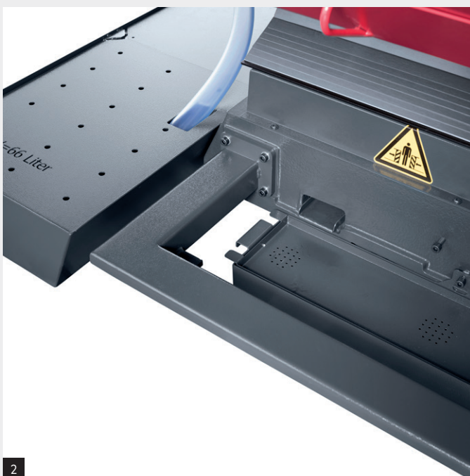
Manual handwheel of X axis (1), Oil dripping pan and coolant tank (2), Splash guard (3)
