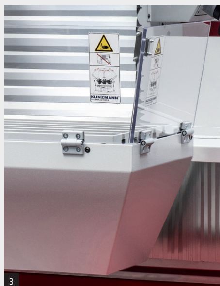
Manual handwheel of X axis (1), Oil dripping pan and coolant tank (2), Splash guard (3)
